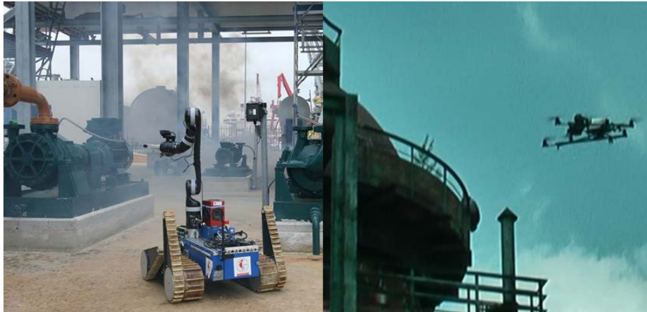
Figure 1: Unmanned Ground Vehicle (UGV; left) and Unmanned Aerial Vehicle (UAV; right) during a field evaluation in the TRADR-project.
